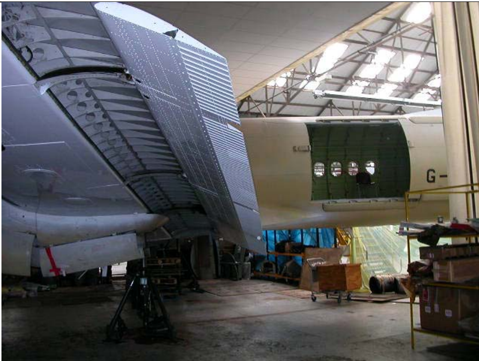
Picture taken Nov 2006 before the Class E was finished . Large Freight door installed
